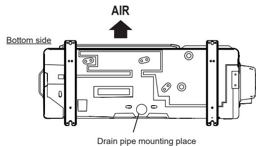
Since the drain water flows out of the outdoor unit during heating operation, install the drain pipe and connect it to a commercial 16 mm hose. (Reverse cycle model only)
