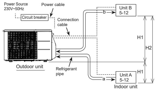
● **Connectable indoor unit capacity type**
